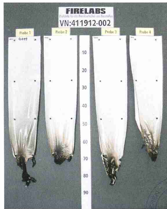
fig. 4 View of test specimen after the test
